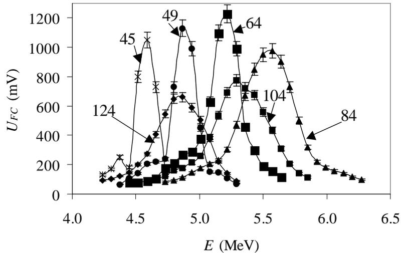
Energy spectra on phase difference between RF gun and pre-accelerator
