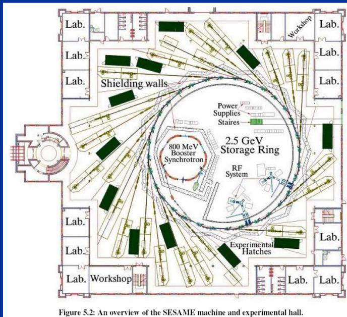
Figure 5.2: An overview of the SESAME machine and experimental hall.
