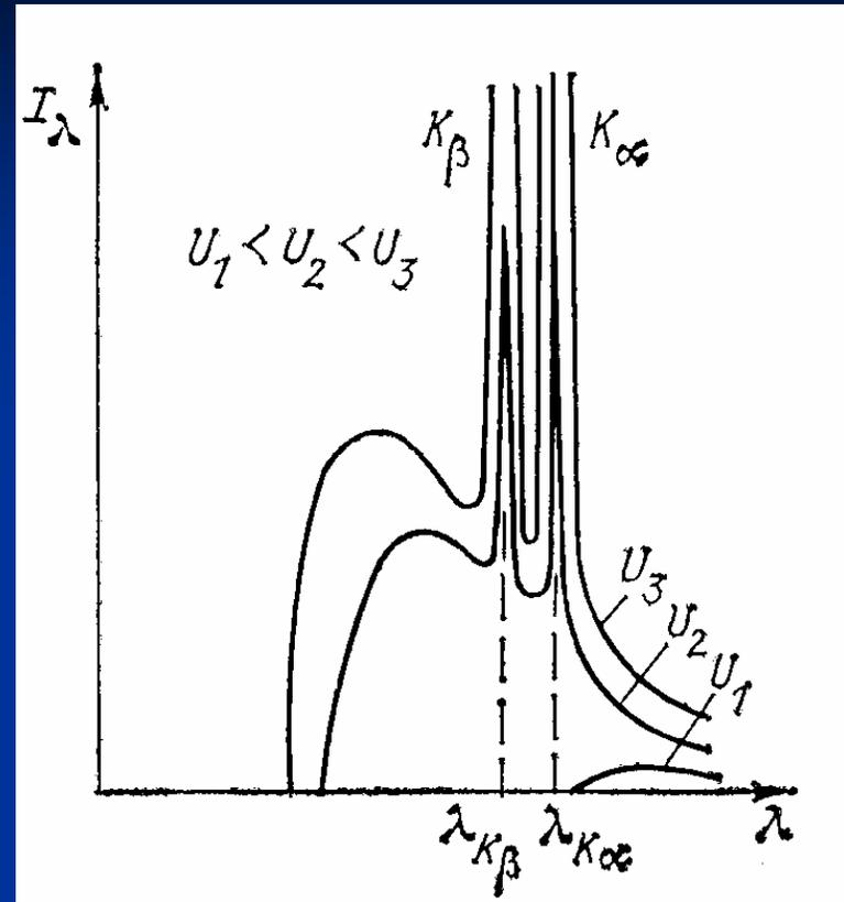
Since 1895. Compact, low cost, robust, but only less than 1% of electron beam energy is transformed to X-ray energy, which is ~uniformly distributed over angles. Energy spectrum is continuous. Heat loading limits attainable brightness. The maximum x-ray tube brilliance is achieved with a rotating anode microfocus x-ray generator at about  $10^9$  photons  $s^{-1}$   $mrad^{-2}$   $mm^{-2}/0.1\%$  BW.
