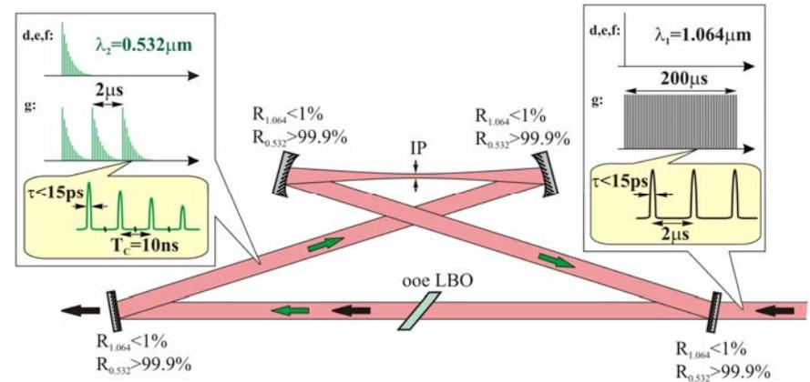
**Fig. 1. Optical circulator based on intracavity Pockels cell.**
