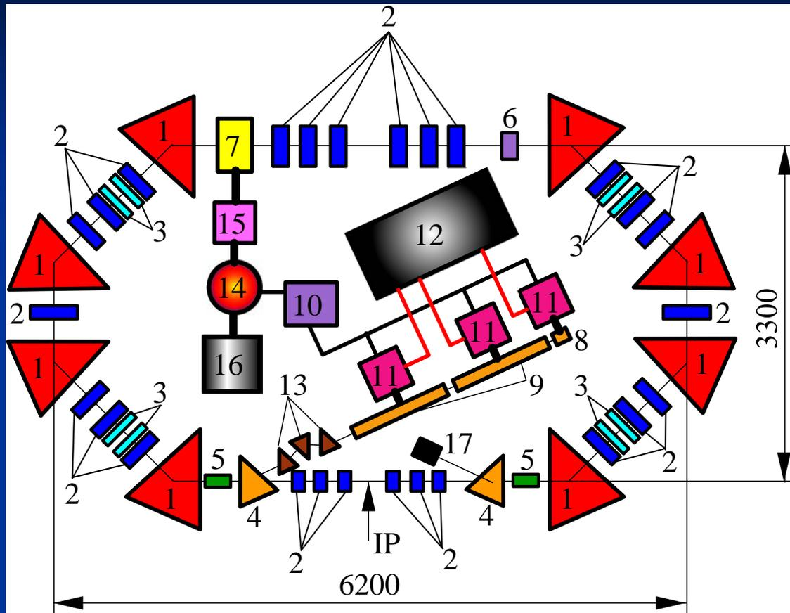
1 – dipole magnets, 2 - quadrupoles, 3 - sextupoles, 4 – septums, 5 – kickers, 6 - beam monitors, 7 – RF cavity, 8 – RF gun, 9 – accelerating structure, 10 – master oscillator, 11 – RF units, 12 – high voltage modulator, 13 – beam stretcher, 14 – klystron, 15 – waveguide elements, 16 – high voltage power supply.
