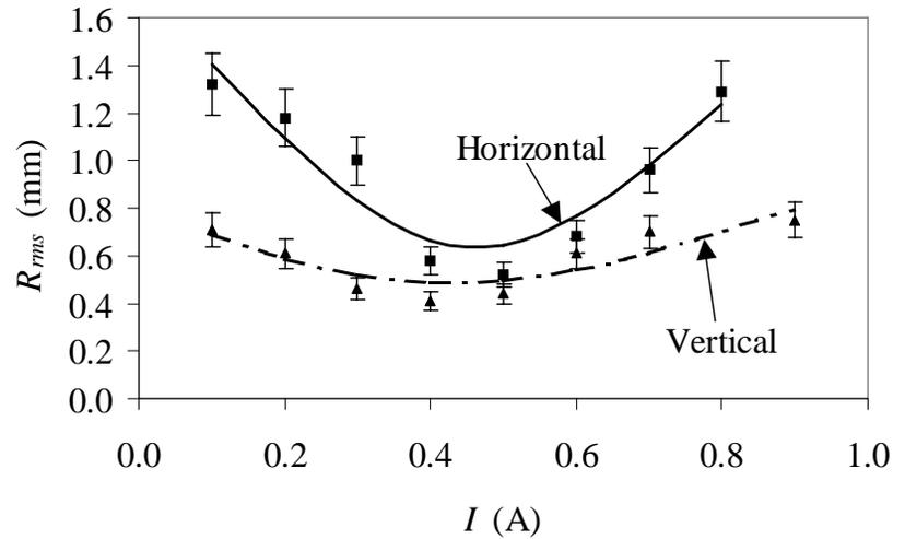
Rms beam radius on focusing lens current, normalized rms emittance,  $8.2 \pm 4$  mm mrad
