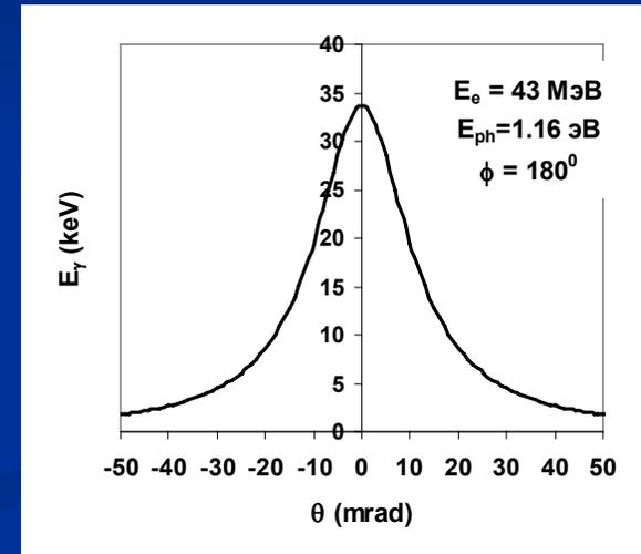
$$E_\gamma \approx \frac{2\gamma^2 E_{ph}}{1 + \gamma^2 \theta^2} (1 - \cos \phi), \quad \gamma \gg 1, \quad \theta \ll 1$$
