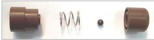
*Gas-gun with 2-piece sabot to protect target*
