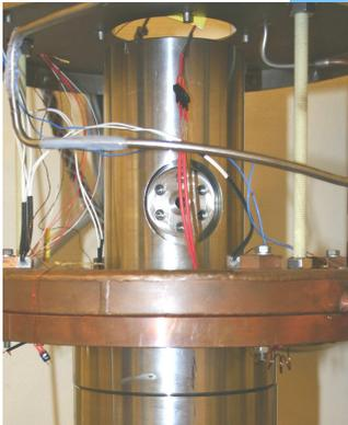
Stirling device + triple cryogenic loops with He under 20 bars)
