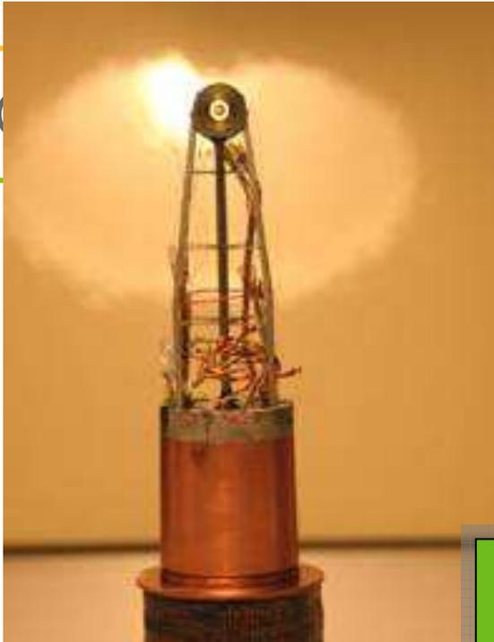
Cryogenic Target Assembly (CTA)
