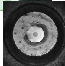
Top view of an anti-convective membrane on a gold ring
