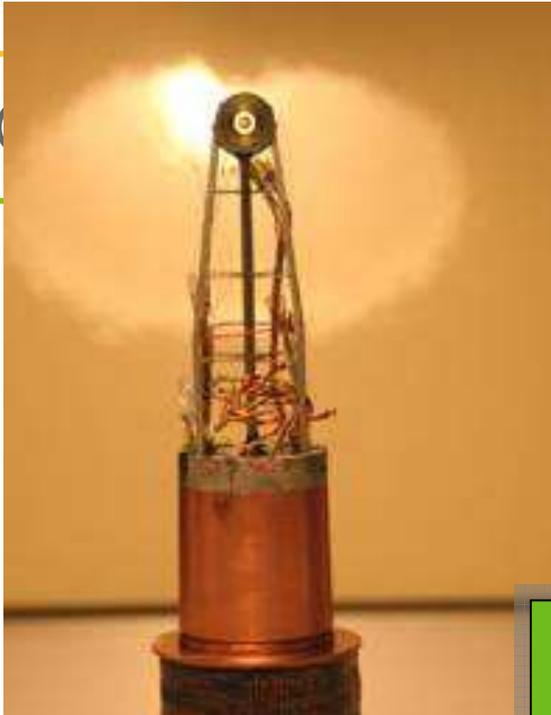
Cryogenic Target Assembly (CTA)
