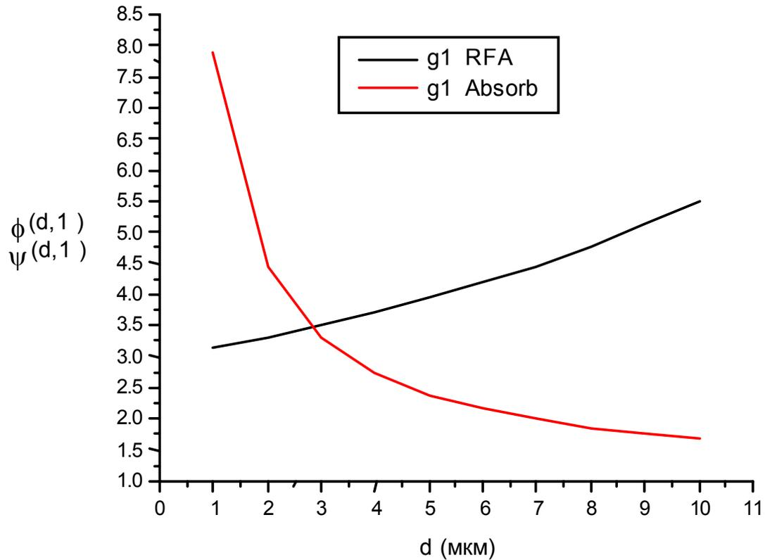
Dependence of a relative error for film thickness measurement by fluorescent and absorptive methods
