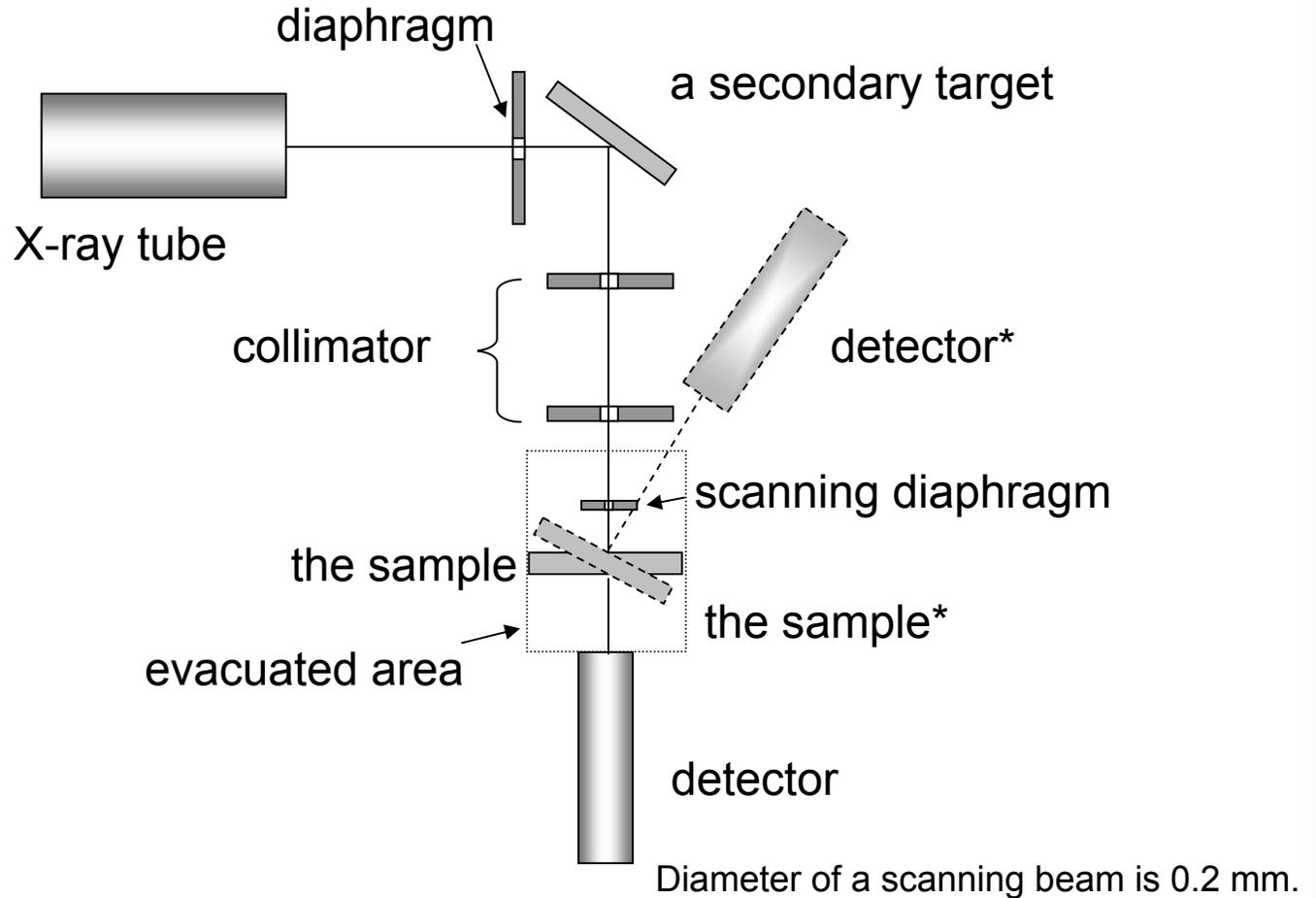
The scheme of film parameters measurements by X-ray absorptive and fluorescent methods
