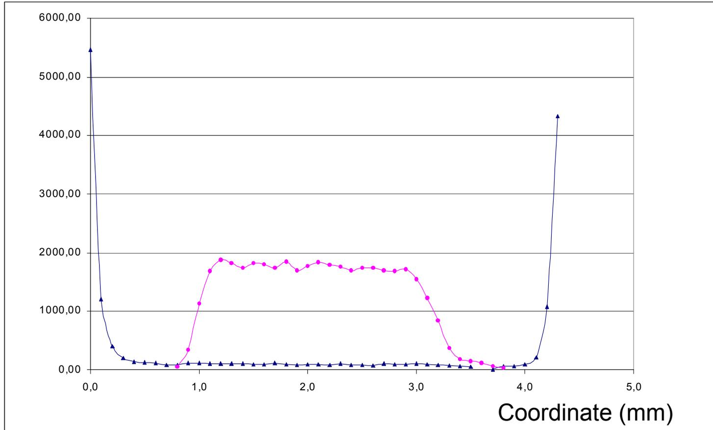
Fluorescence intensity of lead film (the top curve)
