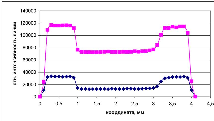
Intensity of quantum of characteristic radiation of a secondary target, past through the Pb-Al sample, versus scanning coordinate.
