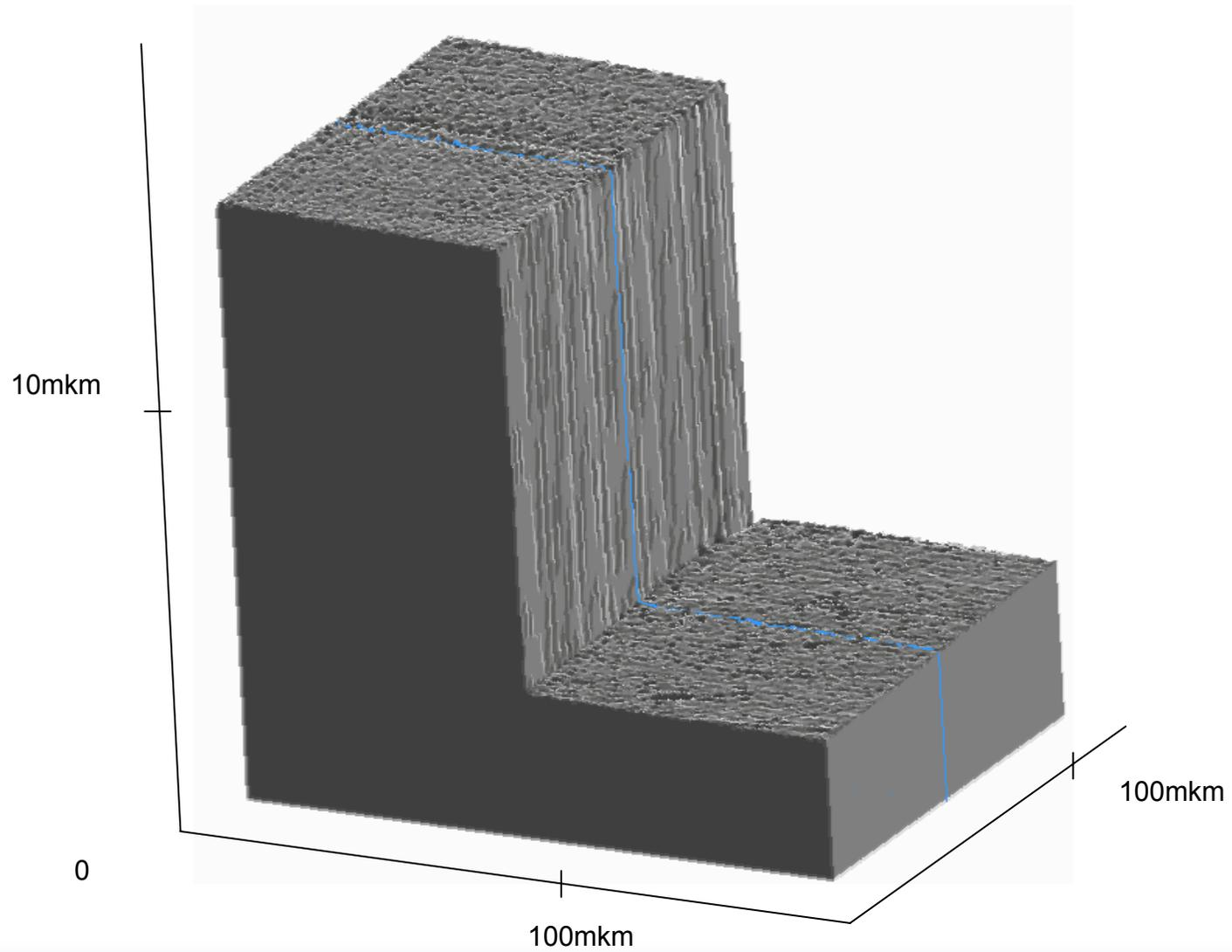
3D images of steps on Al foil, made by means of two-level matrixes
