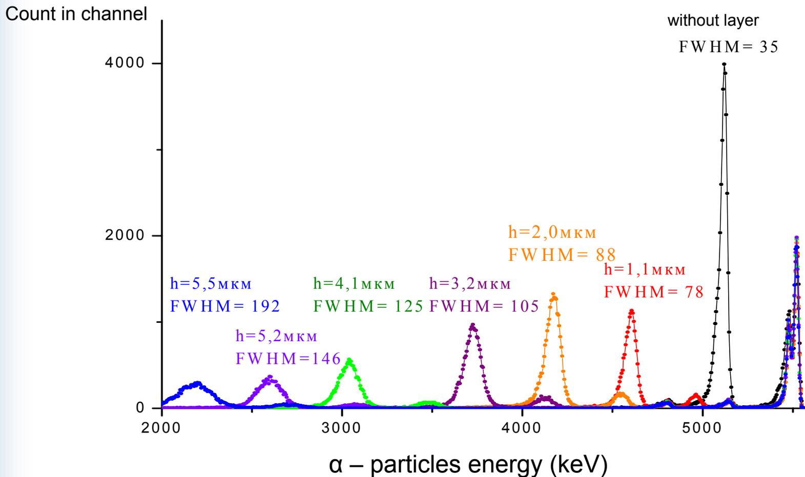
Instrumental spectra at copper film measurement
