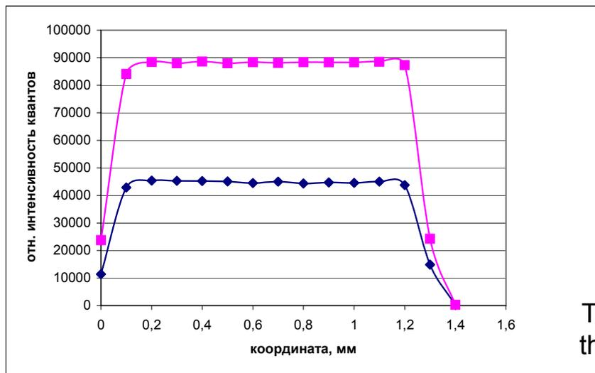
Intensity of quantum of characteristic radiation of a secondary target past through the Cu-Al sample versus scanning coordinate.
