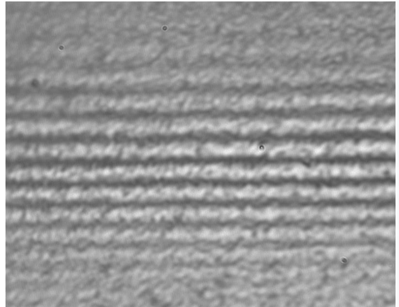
Surface profile of an aluminum layer thickness 12,6 microns on NaCl substrate, measured with AFM.
