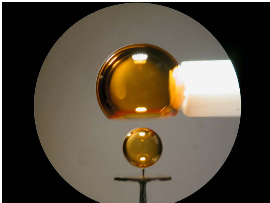
Precision Assembly of a Double Shell Target
